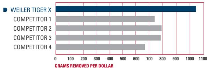
**Test Procedure:** Weiler Tiger X 4-1/2" Type 29 standard density flap disc vs. similar competing flap discs. Test grinder mounted at 15° angle against 1/2" workpiece with 15 pounds of pressure. Bi-directional 8" travel. Discs and workpiece weighed after 5 minutes of operation for life of product. Tiger X usable life: 100 minutes. Competitors' usable life: 65 - 90 minutes.
