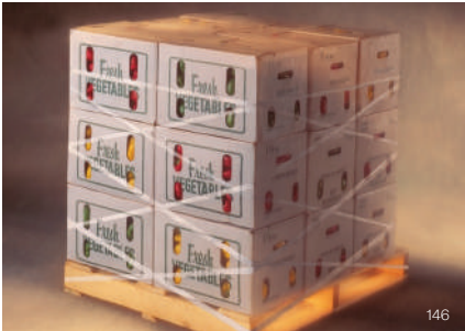
“X”-pattern can contain loads for shipment anywhere.
