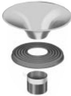
Bonding Voice Coil to Spider to Cone
