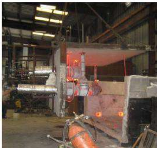
Figure 4-2 Test Assembly Being Moved From the Furnace (approximately 1 or 2 minutes after termination of the test)
