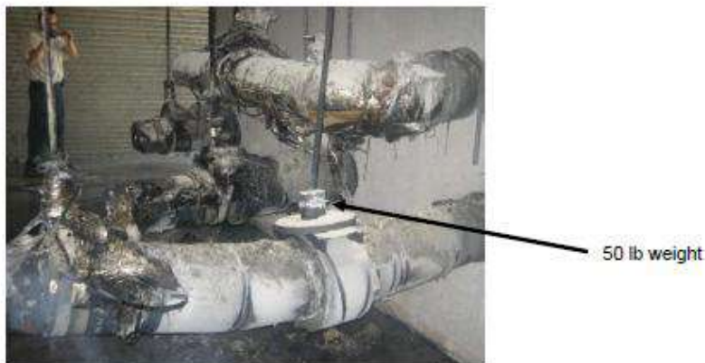
Figure 4-12 Specimen C Following Hose Stream Test
